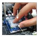
Remove the cap from lever hinge side (as the arrow shows). The pins of socket reveal.
